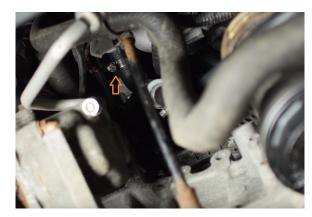
11. Tighten the clamps at all connections.
