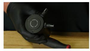
Install the catch can to the bracket and secure it with the provided hardware from your kit. (2x M4 screws and washers)
