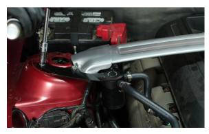
The contents of the catch can should be checked and drained every 1000 miles until a baseline for oil accumulation is established. The volume collected in the can will be different for every car and will vary based on climate, temperature, and driving conditions.
