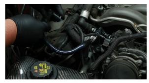
4. Thread the two plastic fittings from your kit onto the catch can.
