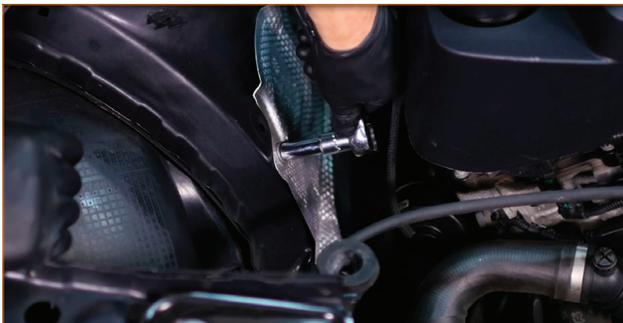
14. Lower the catch can assembly into place over the strut tower, and secure it with the hardware you just removed. Then go back and tighten the two bolts that secure the support strut to the catch can bracket. (2x 13mm bolts, 1x 10mm screw)
