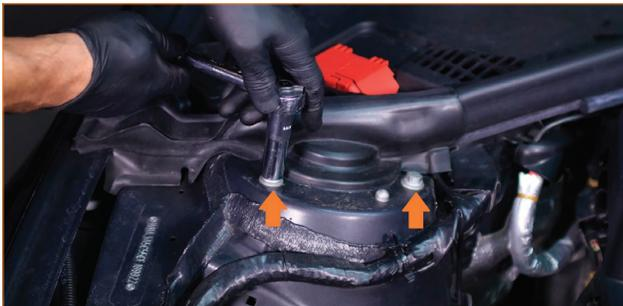
13. Remove the screw that secures the top of the heat shield below the passenger-side strut tower. (1x 10mm screw)
