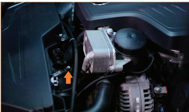
07. Remove the airbox from the vehicle by lifting it upward. The airbox is held in by three pegs and grommets.
