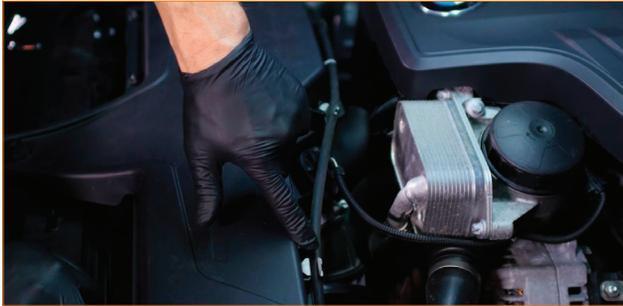
05. Disconnect the wiring harness from the mass airflow (MAF) sensor. To release the connector, depress the black tab.
