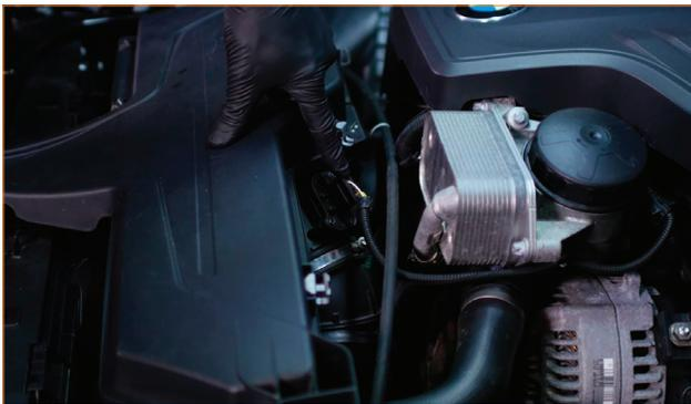
06. Loosen the clamp that secures the intake hose to the MAF housing. Then separate the hose from the MAF housing. (1x worm-gear clamp)
