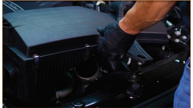
08. Locate the CCV hose attached to the front of the engine. Disconnect the hose from the valve cover by squeezing the tabs at the top of the hose and pulling the hose off. Then disconnect the wiring harness from the sensor at the other end of the hose. Separate the bottom of the hose by squeezing the tabs and pulling the hose off.
