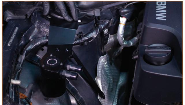
15. Locate the hose with the smaller bend, and install one of the provided hose clamps over the wider end. Install this end to the CCV fitting on the valve cover. Attach the other end of this hose to the fitting marked **IN** on the catch can. (1x worm-gear clamp)
