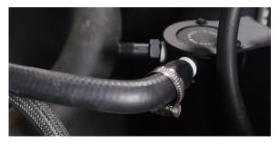
14. Slide a clamp over the shorter, straight hose and connect it to the IN port on the intake manifold. (1x worm gear clamp)
