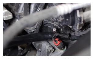
15. Slide a clamp over the other end of the hose and install it onto the catch can's OUT port.(1x worm gear clamp)
