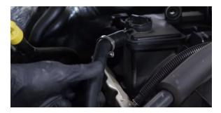
13. Slide a clamp over the other end of the hose and install it onto the catch can's IN port.(1x worm gear clamp)
