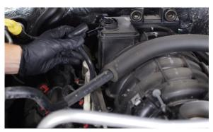
6. Separate the PCV line from the IN port on the intake manifold and remove the PCV line.
