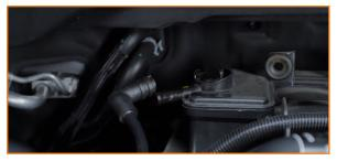
3. Release the tab on the clip that holds the PCV hose. Then remove the hose from the engine bay.
