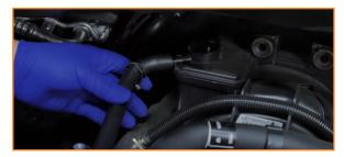
Install the smaller hose to the intake port. (1x worm gear clamp)
