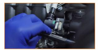
4. Feed the longer hose under the intake and connect it to the PCV valve housing.(1x worm gear clamp)
