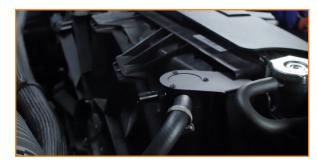
12. Connect the shorter hose to the outlet port on the catch can. (1x worm gear clamp)
