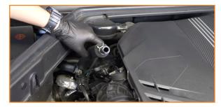
2. Slide the provided aluminum spacer over the adjacent M6 stud.
