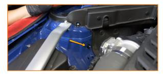
3. Loosen the nut on the passenger side strut tower, just above where you placed the spacer. Install the catch can bracket under the loosened nut as shown here. Secure the bottom of the bracket at the M6 stud. (1x 10mm nut, 1x 14mm nut)
