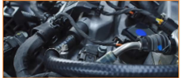
25. Attach the other end of the hose from the valve cover to the inlet port on the catch can. (1x worm gear clamp)
