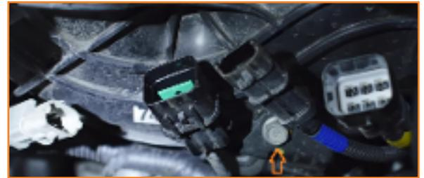
5. Remove the bolt on the bracket that holds the coolant line to the intake manifold. (5x 10mm bolts)
