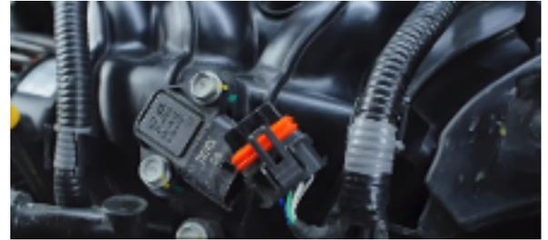
4. Remove the bolt on the bracket that holds the bottom sensors. (1x 10mm bolt)
