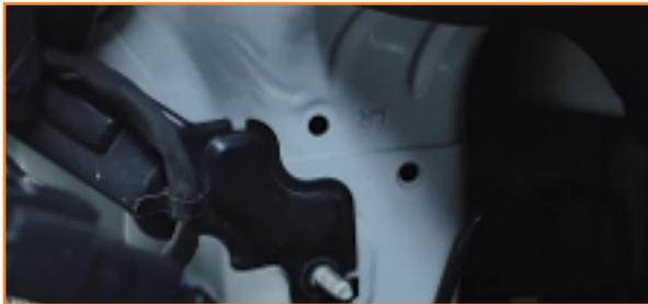
21. Place the catch can bracket over the studs. Secure it with the provided hardware. (2x 10mm nuts)
