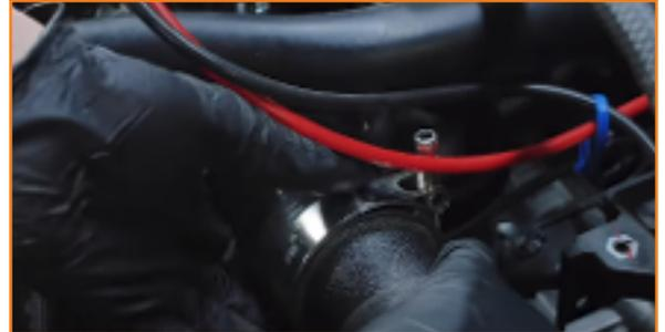
11. Slide the intake manifold forward to reach the clamp on the PCV hose.
