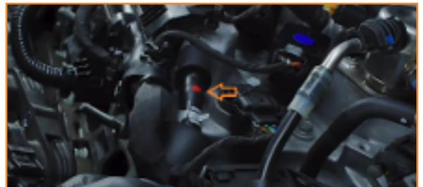
13. Feed the longer hose from your kit to the intake manifold port. Use the straight end for this step. (1x spring clamp)
