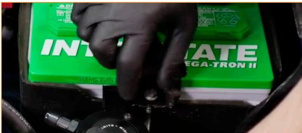
12. Locate the hose with three bends in your kit. Lead the end with the 90° bend under the electrical harness and AC lines as shown here. Slip a worm-gear clamp over the end of the hose and install it to the CCV port on the engine. Now tighten the clamp to secure the hose. (1x worm-gear clamp)
