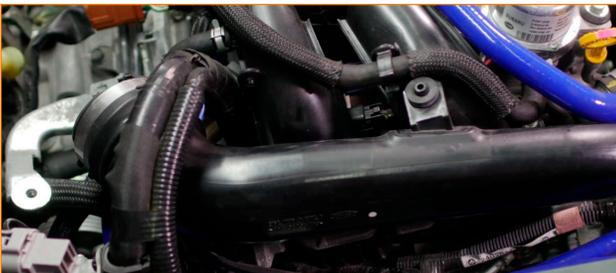
35. Now tighten the bolts that secure the catch can to the bracket.
