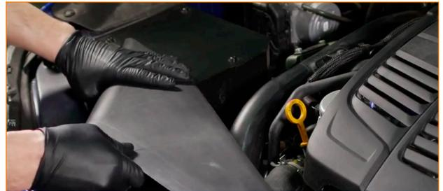
03. Remove the two pop-clips that secure the back of the plastic engine cover. Then remove the engine cover from the vehicle by lifting it from the front edge. The front edge is held on with two pegs and grommets. (2x pop-clips)
