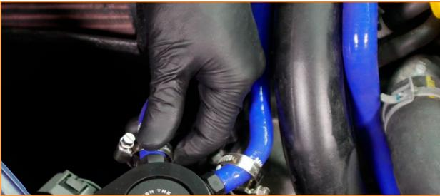
34. Check the routing on your hoses. The hose connected to the IN port on the catch can should be attached to the PCV valve on the engine block. The hose connected to the OUT port on the catch can should be attached to the port on the intake manifold.
