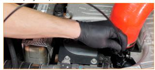
05. Locate the straight hose included with your kit. Slip a worm-gear clamp over one end of the hose and attach the hose to the crankcase vent on the driver-side valve cover. Then tighten the hose to secure it. (1x worm-gear clamp)
