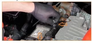
10. Install the catch can mounting bracket over the EGR cooler and secure it with the provided Allen bolts. (2x 5mm Allen bolts)
