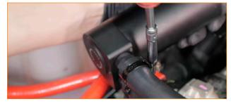
09. Remove the two bolts that secure the EGR cooler bracket to the engine. (2x 10mm bolts)
