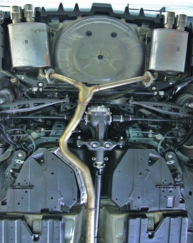
FIGURE 3: Stock exhaust. Notice the single entrance and dual-tip design. Stock mufflers will cause more backpressure and also detain more sound.
