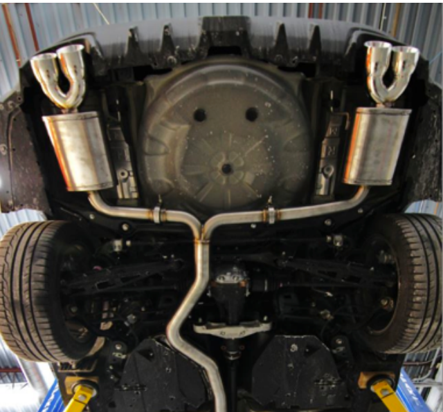
FIGURE 4: Mishimoto exhaust. Notice larger pipe diameters and the straight-through design of the mufflers. This reduces unwanted backpressure.
