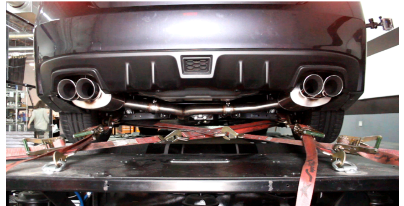
FIGURE 6: Eye-level view of the Mishimoto exhaust while strapped to the dyno during a performance testing cycle.
