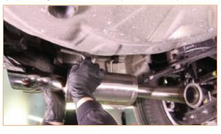
5. Install the band clamp exhaust onto the mid-pipe. Make sure the hardware faces the driver side.
