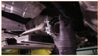
**6.** Spray the rubber exhaust hanger with WD-40 and attach to the Y-pipe.
