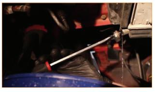
4. Remove the two pop clips on the fan shroud.
