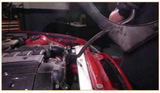
**16.** Install the rubber bushings onto the Mishimoto fan shroud. (4x bushings and 2.5mm Allen bolts)
