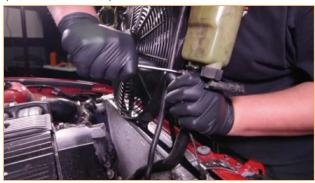
**19.** Install the supplied bracket for the stock expansion tank. (2x 10mm bolts)
