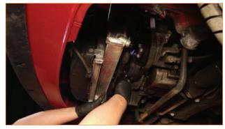
**25.** Reinstall the air dam using the Phillips head screws and pop clips removed in **step 1.**
