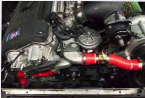
Figure 2: Mounting locations for temperature sensors, which read approximately 10 times per second.
