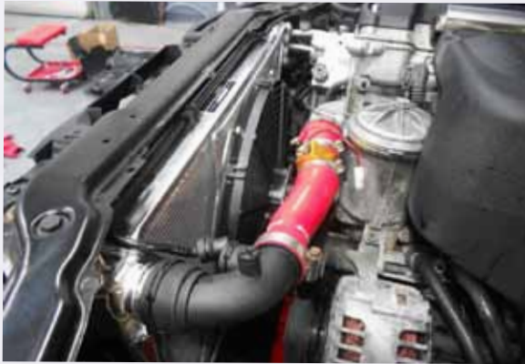
Figure 4: A 16" electric fan was installed with the Mishimoto radiator.
