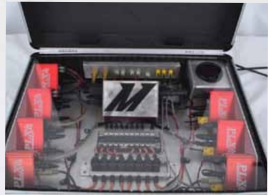
Figure 3: PLX sensor modules were used to monitor engine pyrometers.
