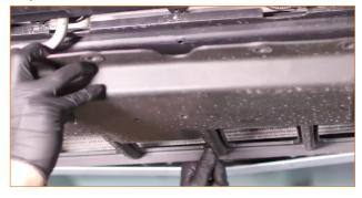
08. If equipped, remove the four nuts that secure the stock HD oil cooler to the underside of the vehicle. Slide the oil cooler off of the studs in order to access the petcock on the radiator. (4x 10mm nuts)
