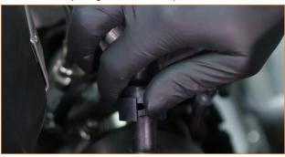
04. Disconnect the mass airflow (MAF) sensor and release the harness from the intake tubing. To release the connector, slide the red locking tab up, depress the black tab and pull the connector off the sensor.
