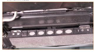
09. Place a drain bucket underneath the petcock on the radiator and use a pair of pliers to open the petcock. Remove the pressure cap from the expansion tank to expedite the draining process. Close the petcock on the radiator once all the coolant has drained.
