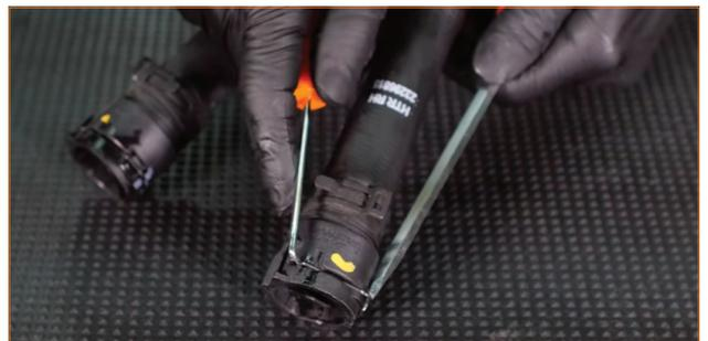
13. Compress the clamps that secure the quick-disconnect fittings to the factory hoses and remove the fittings. Lubricate the fittings with fresh coolant and transfer them to the Mishimoto heater hoses. Orient the fittings so the clip will be easily accessible when installed on the car and secure them with the provided hose clamps. (2x spring-clamps, 2x worm-gear clamps)
