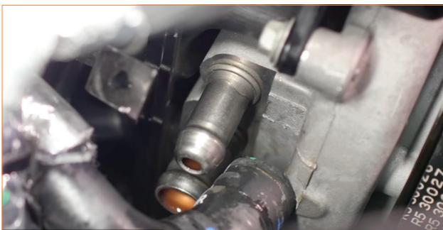
11. Compress the clamp that secures the heater hose to the back of the expansion tank and separate the hose. (1x spring-clamp)
