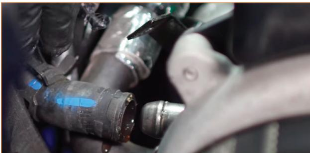
10. Separate the tree-clip that secures the lower heater hose to the engine. Then compress the clamp that secures the lower hose to the water pump, and separate the hose. (1x spring-clamp, 1x tree-clip)
