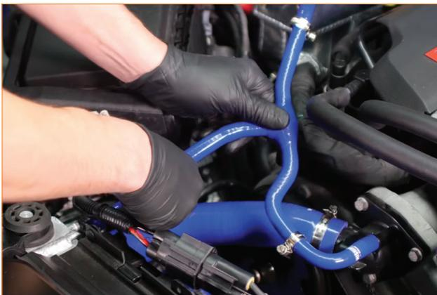
18. Fill the cooling system with premixed, Chevy-approved coolant, start the engine, and allow it to idle with the cap off. Turn the heater control valve on the vehicle's HVAC unit to full hot, and put the fan on low. Monitor the engine temperature and coolant level in the reservoir. Add coolant as needed to maintain proper level in the reservoir, and
