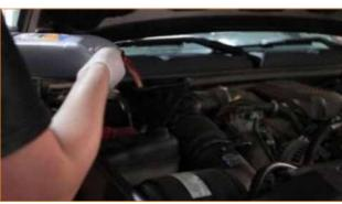
**7.** Start the vehicle and set the heat to high to purge the cooling system of any air bubbles. Allow the vehicle to reach operating temperature and check for any leaks.
