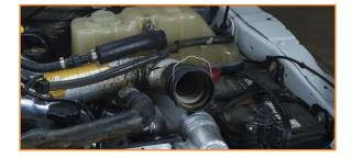
3. Pull the clip from the other end of the radiator hose and separate the connection. (1x spring clip)
