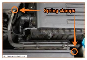
2. Remove the stock coolant hose from the driver side of the radiator. (2x spring clamps)
