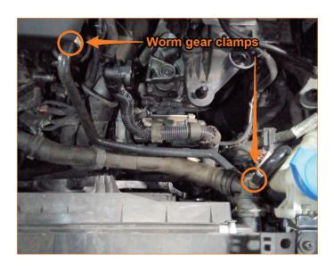
\*The image above shows the Mishimoto coolant hose routing with the air box removed\*
