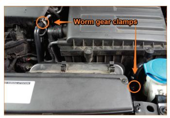
3. Route the Mishimoto coolant hose under the air box ducting, then secure it in place using the provided worm gear clamps.
