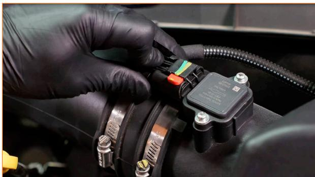
02. Loosen the clamp that secures the stock intake hose to the airbox. (1x worm-gear clamp)
