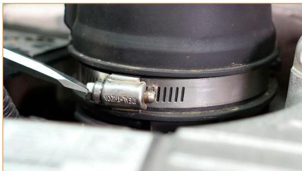
04. Remove the intake hose from the vehicle by pulling it off the turbocharger inlet and airbox.
