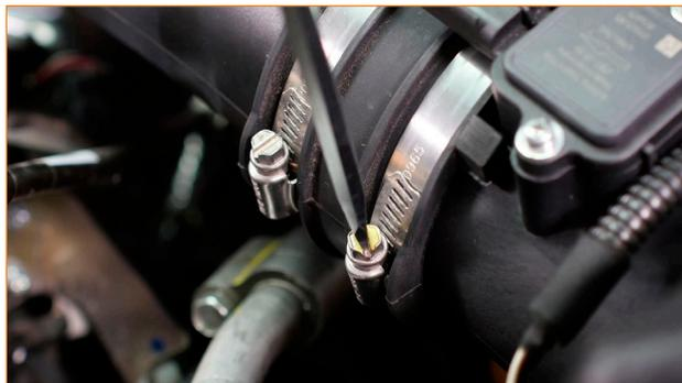
03. Loosen the clamp that secures the intake hose to the turbo charger inlet. (1x worm-gear clamp)
