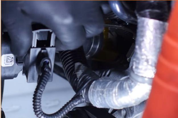
12. Reach down through the engine bay on the passenger side, and use a pick to lift the circlip on the cold-side pipe until it locks into the detent, as shown here. This detent will hold the circlip in the unlocked position.
