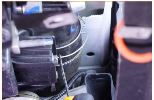
16. Remove the hot-side pipe from the vehicle. The pipe can be separated into two pieces by loosening the worm gear clamp. To remove it in one piece, slide it back toward the firewall, and feed the intercooler connection past the turbo first.
