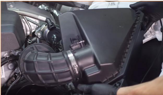
06. Remove the five screws that secure the air diverter to the driver side of the vehicle, and remove the air diverter. Repeat this process on the passenger side. (10x 7mm screws)
