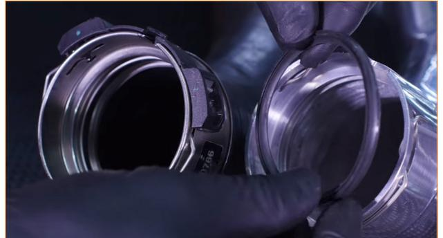
20. Lower the cold-side pipe into place, and slide the quick-disconnect fitting over the intercooler outlet until it locks. You will hear an audible click when the circlip drops into the channel on the intercooler.
