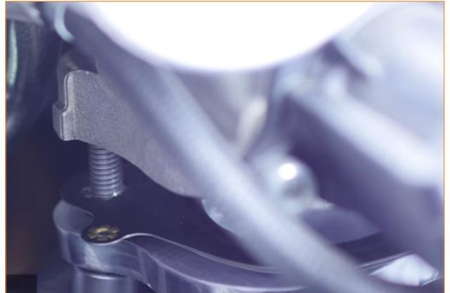
29. Adjust the coupler on the hot-side pipe so that both sections are engaged, and then tighten the clamps to secure the coupler.
