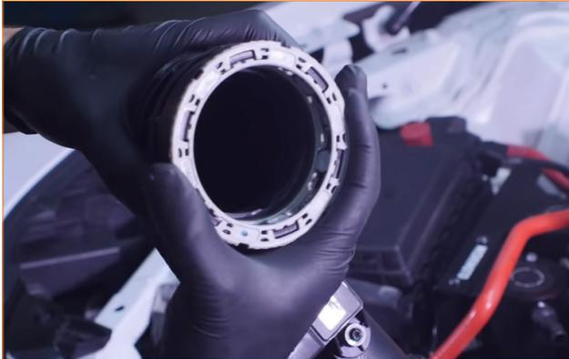
18. Remove the screw that secures the sensor to the cold-side pipe. Then remove the sensor by pulling it directly outward. Transfer the sensor to the Mishimoto cold-side pipe, and secure it with the provided bolt. Do not reuse the original screw on the Mishimoto cold-side pipe. (1x T20 screw, 1x 10mm bolt)
