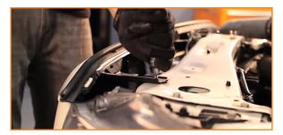
Remove the bolts on the front grille mounting points. Next, disconnect the fog light harness and remove the hardware.
