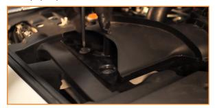
5. Remove the bolt that secures the airbox. Loosen the clamp where the intake hose meets the airbox. Then remove the airbox from the engine bay. (1x 10mm bolt, 1x 10mm clamp)
