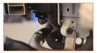
17. Unbolt the lower intercooler pipe from the airbox mounting plate. The entire airbox mounting plate for this step can be removed to make the installation easier but is not required. (1x 12mm bolt)
