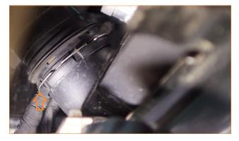
Loosen the clamps that secure the hot-side pipes to the intercooler. Then wiggle the pipes to break them loose from the intercooler. (2x worm gear clamps)
