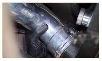
38. Locate the transition coupler included with your kit. Install an 89–97mm clamp over the wider end of the coupler and a 79–87mm clamp over the smaller end.
