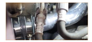
28. Align the driver-side intercooler pipe with the lower inlet of the intercooler, and slip the coupler down to join the connection.
