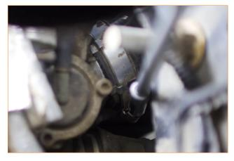
09. Reach through the driver-side wheel well and loosen the clamp that secures the hot-side pipe to the turbocharger. (1x worm gear clamp)
