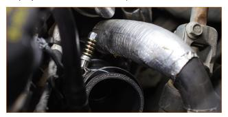
18. Locate the upper section of the driver-side intercooler pipe. Lead the end with the shorter run of pipe underneath the hoses at the front of the engine bay, and turn the pipe so that the other end runs across the front of the engine. Then slip the pipe into the coupler at the turbocharger.
