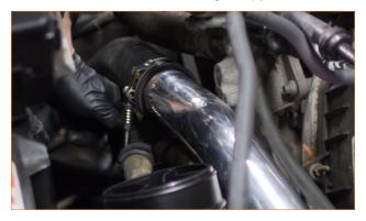
**32.** Tighten the clamp that secures the passenger-side turbocharger coupler to the intercooler pipe. Then secure the passenger-side induction pipe to the engine by pushing the pin on the pipe into the grommet on the engine.
