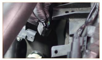
**06.** Disconnect the hose from the cold-side intercooler pipe. To release this connection, squeeze the tabs on the underside of the connector, and slide the locking clip away from the port.
