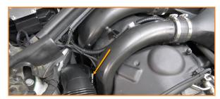
7. Disconnect the MAF sensor. Depress the black tab at the center to release the connection. Then lift the airbox out of the way.
