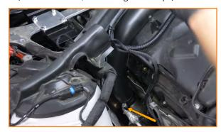
14. Attach a silicone coupler to the front intercooler pipe. Then set the front pipe and slide the coupler onto the intercooler.(1x E11 torx bolt, 2x worm gear clamps)
