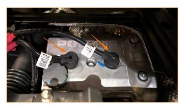
**06.** Loosen the 2X T-bolt clamps holding the factory charge pipe to the turbo outlet and the throttle body. Loosen until the nut reaches the end of the T-bolt for easiest removal.
