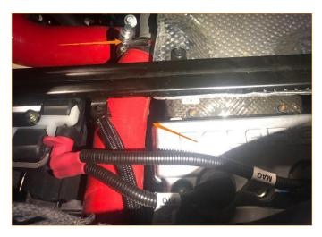
11. Using a T-20 Torx, remove the MAP sensor from the outlet side of the factory charge pipe. Install the MAP sensor in the sensor fitting of the charge pipe. Secure with the provided bolt using a 3mm allen key. The MAP sensor fitting may need to be adjusted slightly by rotating it in place. Re-install MAP sensor and throttle body electrical connections.
