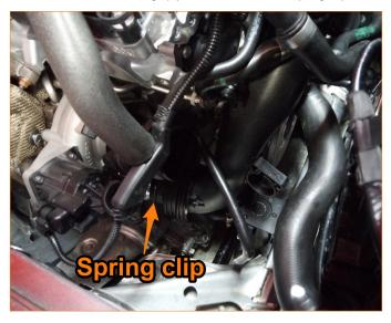
06. Remove the stock charge pipe from the throttle body.(2x T30 Torx bolts)
