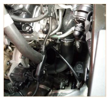
**11.** Connect MM2362-02 loosely to MM4551-01 using one of the provided constant tension worm gear clamps, then connect MM2362-02 to the throttle body. (1x MM1533-92 and 2x T30 Torx bolts)
