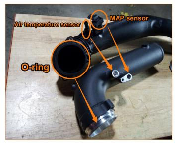
**09.** Swap the turbo side o-ring and the spring clip to MM2362-01.
