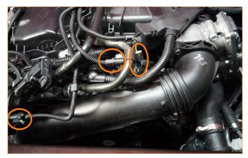
04. Remove the electric water pump from its mounting bracket.(1x 10mm nut)
