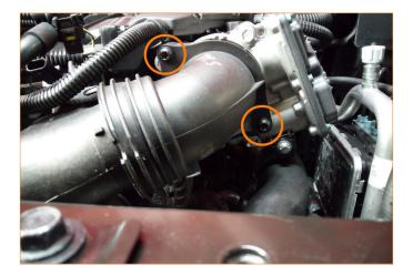
07. Remove the stock charge pipe from the vehicle.
