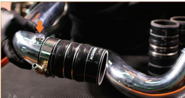
08. Slip one of the provided T-bolt clamps over each end of the short boot and install it to the cold-side intercooler pipe. (2x 10mm T-bolt clamps)
