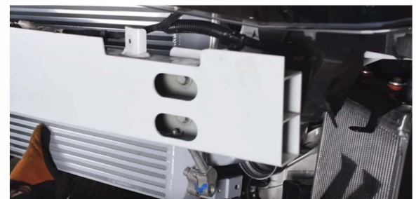
31. Lower the stock intercooler from the vehicle. 32. Install the Mishimoto intercooler by lifting it up into the same location as the stock component and letting it rest on the lower brackets. The AC condenser was removed for this image to give a better view of the step, but you can still install the part without removing the condenser.
