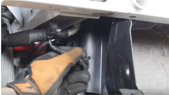
26. Remove the radiator stay ends and upper shroud. (4x 10mm bolts)
