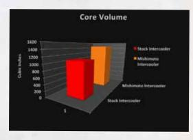
The engineering team went through multiple iterations while designing the end tanks. They used CFD software to make sure that the flow was optimized for the Chevrolet/GMC 6.6L Duramax. The core of the Mishimoto intercooler is 23% thicker and 25% larger in volume than the stock unit.
