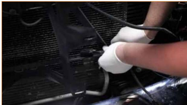
22. Reinstall the clips on the cold-side intercooler pipe and install the pipe on the intercooler and intake manifold.
