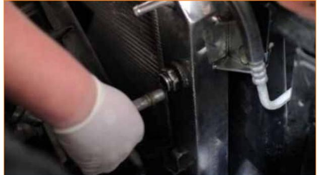
5. Place the upper fan shroud over the radiator assembly.
