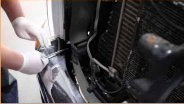
16. Disconnect the electrical connections located on the hood latch support.
