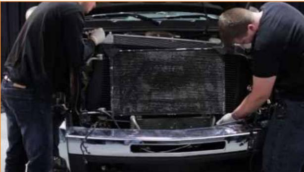
2. Reinstall the upper radiator support beam. This beam is held in place with six 10mm bolts.
