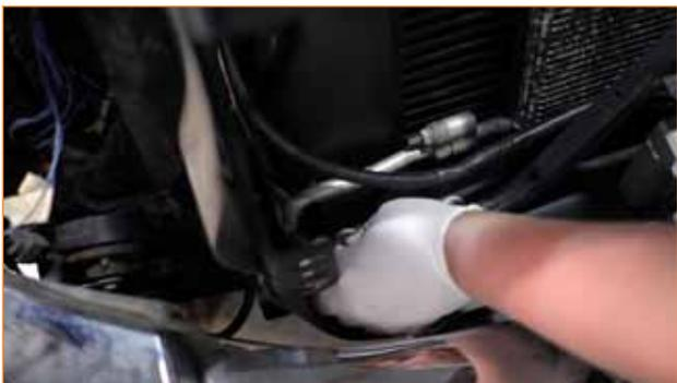
17. Install the two 10mm bolts securing the hood release frame to the upper radiator support bracket.
