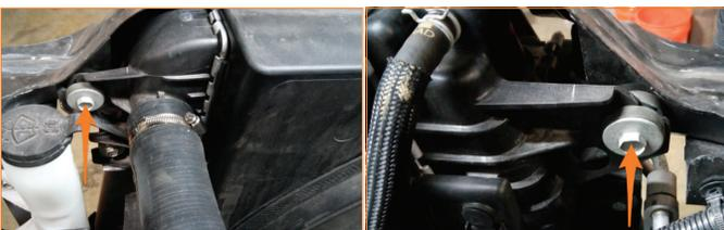
**16.** Remove the bolts securing the radiator to the upper core support. [2x 13mm bolts]
