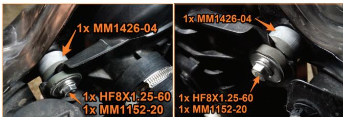
**41.** Using the provided spacers, bolts, and washers, secure the radiator to the upper core support. (2x MM1426-04, 2x MM1152-20, 2x HF8X1.25-60)
