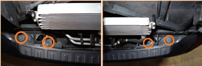
**8.** Remove the front bumper bolts, then remove the bumper from the vehicle. (4x 18mm bolts)
