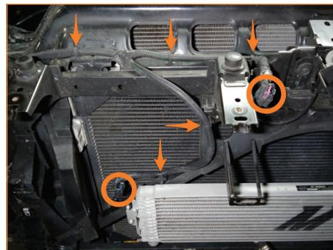
**13.** Disconnect the temperature sensor and hood latch, then unclip the wire harness from the upper radiator support and grille support. (2x electrical connectors, 5x harness routing tree clips)
