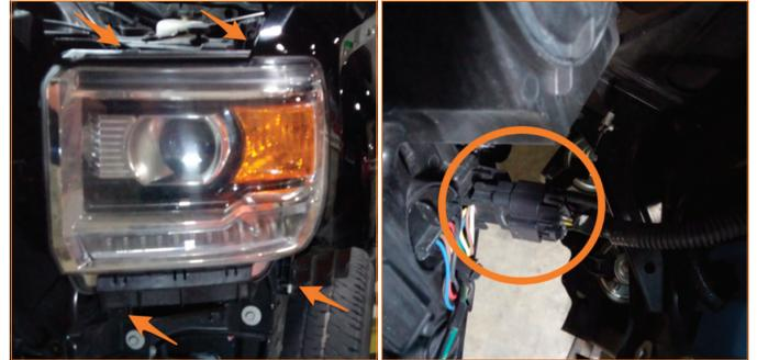
**11.** Remove the headlights. (4x 10mm bolts and 1x electrical connector on each side)
