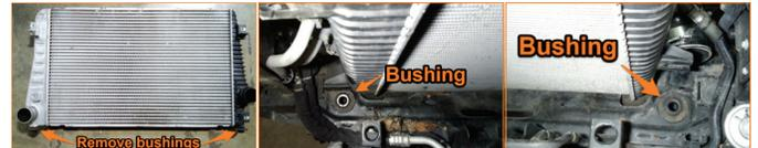
**33.** Remove the bushings from the bottom pegs on the intercooler and reinstall them into their location on the vehicle. (2x bushings)
