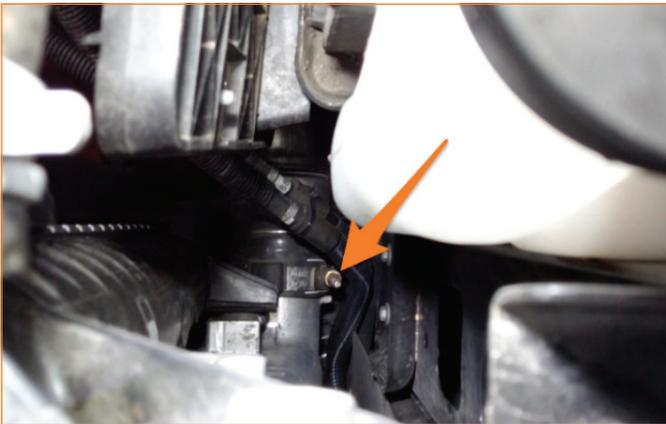
**28.** Disconnect the hot-side intercooler pipe from the intercooler. (1x constant tension T-bolt clamp)
