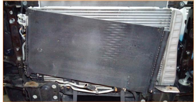
**31.** Unseat the A/C condenser from its lower mounts. Lift the A/C condenser up and over the power steering cooler, then place it back down carefully.
