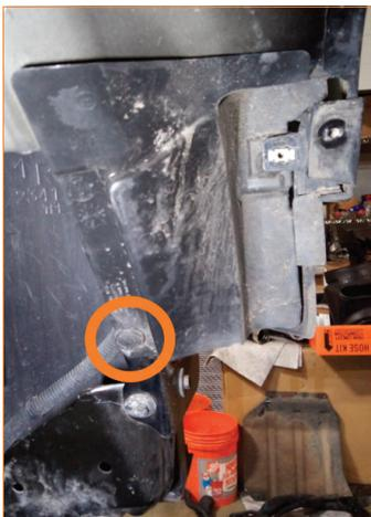
**9.** Remove the plastic cover in the passenger-side wheel well. (1x pop clip)
