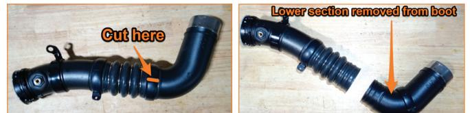
**25.** Cut plastic retaining ring on stock cold-side intercooler pipe lower section and remove the lower section from the boot. Note: Be careful not to cut the boot underneath the plastic retaining ring.
