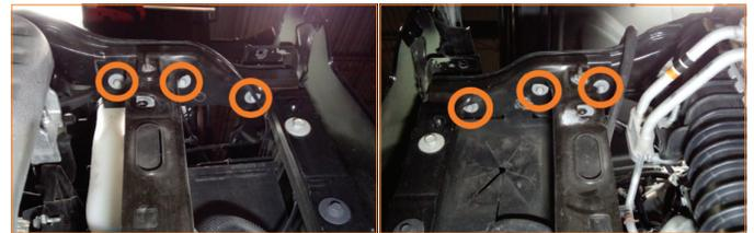
**18.** Remove the upper core support from the vehicle. [6x 10mm bolts]
