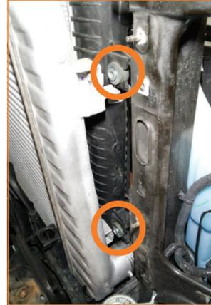
**30.** Remove the grommets from the driver-side brackets on the radiator. (2x grommets)
