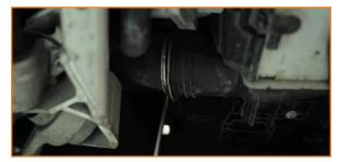
4. Turn the tabs on the intercooler shrouding to release it from the intercooler.
