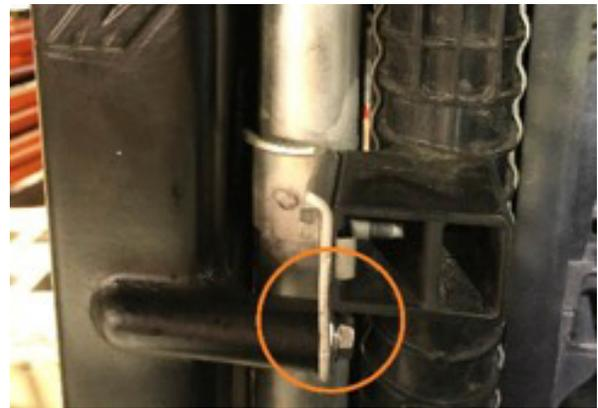
**20.** Trim the foam shrouds with scissors as shown to minimize contact with the Mishimoto intercooler and reinstall with factory clips.
