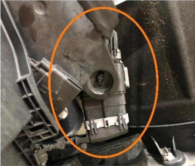
**7.** Remove the fresh air duct from the grille shutter assembly by pulling apart at this junction.
