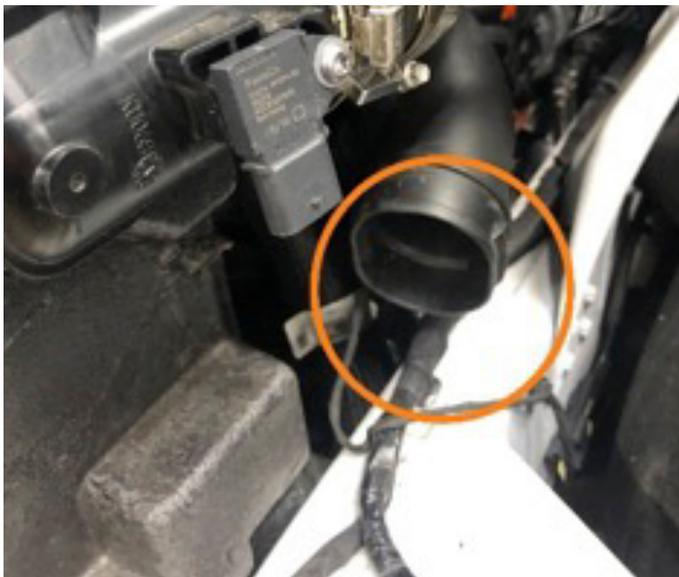
**8.** Remove hood latch cable by un-clipping cover and removing the cable. Move the cable out of the way.
