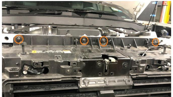
**10.** Remove the 7x 10mm bolts holding the bottom of the grille shutter assembly to the vehicle. If you have a 2020+ model, there may be 6x aluminum rivets instead of the 7x bolts. Drill the 6x rivets out using a 1/4" or similar size drill bit.
