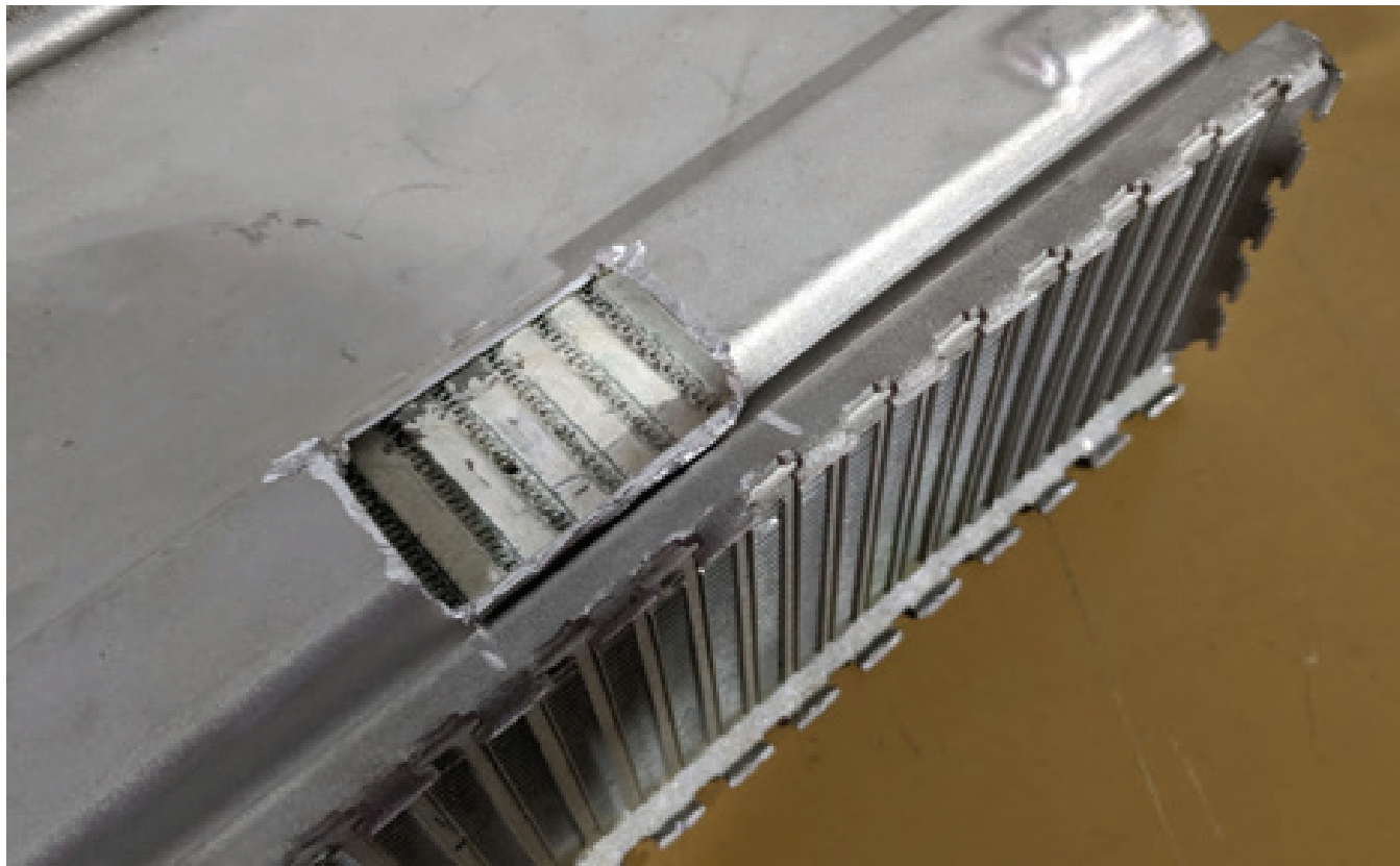
FIGURE 1: The stock intercooler's internal coolant fins and the orientation of the air passages.
