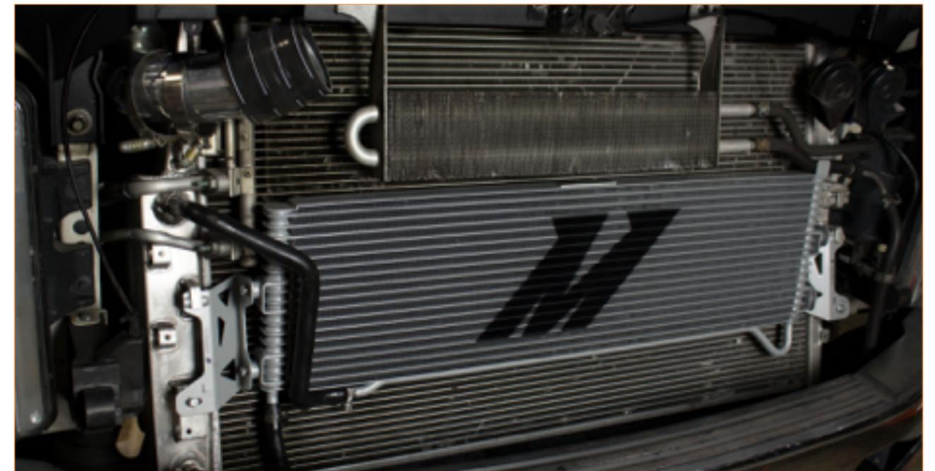
FIGURE 3: Mishimoto transmission cooler installed (intercooler off).
