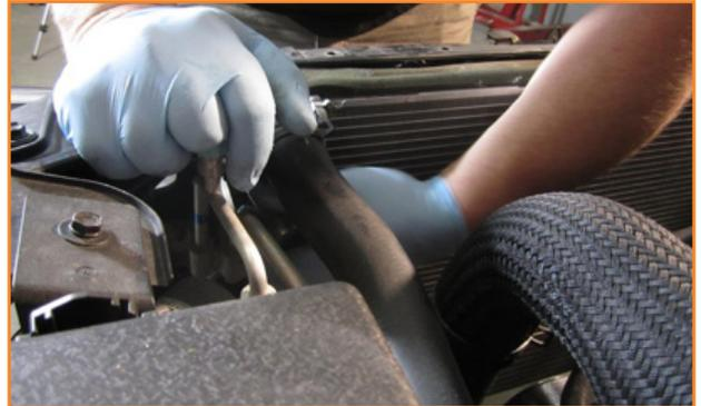
13. Pull off insulator strip on top of radiator.
