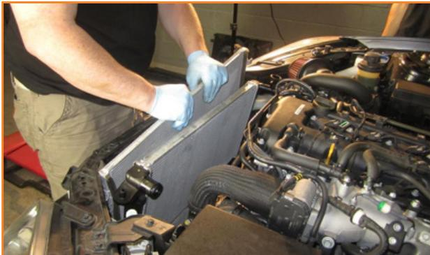
18. Disconnect the Intercooler charge piping.
