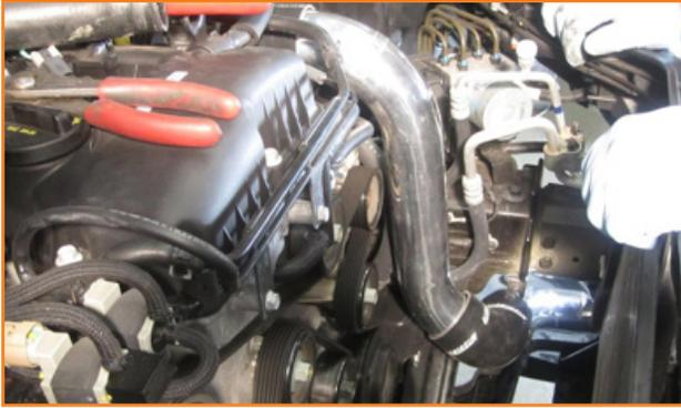
5. Install T-Bolts clamps onto cold side piping.
