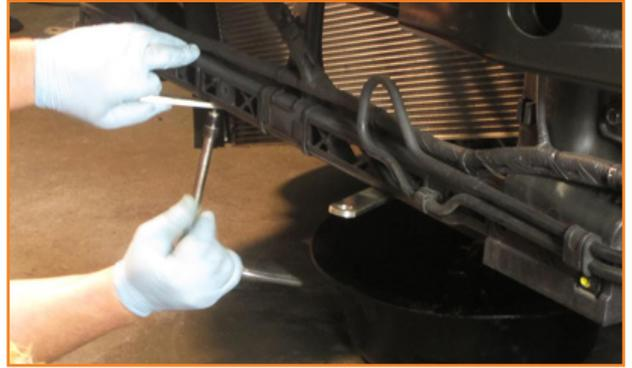
2. Mount the intercooler, tighten M6 x 1.0 bolts, and install the intercooler with the provided (2) M12 x 1.75 x 20mm bolts. Leave loose. Install Mishimoto couplers onto intercooler.
