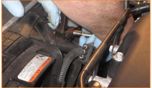
14. Plug fan in and reattach wiring harness onto the fan shroud and reinstall the coolant overflow container and overflow rubber line.
