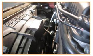
12. Remove (2) 10mm bolts for the A/C condenser.
