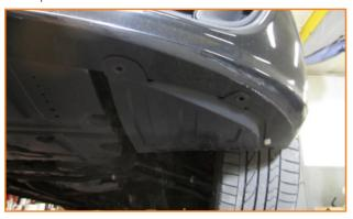
**4.** Remove the (4) plastic screws for the intake dam. Lift up and remove from vehicle.
