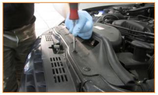
**5.** Remove the (2) screws holding the corner of the bumper onto the fenders.
