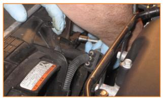
**14.** Plug fan in and reattach wiring harness onto the fan shroud. Reinstall the coolant overflow container and overflow rubber line.
