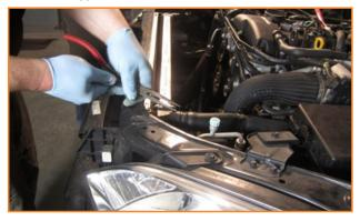
**12.** Reinstall the (2) 10mm A/C condenser bolts and reinstall the insulator strip.
