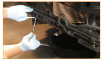
**2.** Mount the intercooler, tighten M6 x 1.0 bolts, and install the intercooler with the provided (2) M12 x 1.75 x 20mm bolts. Leave loose. Install Mishimoto couplers onto intercooler.
