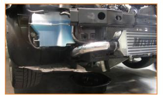
7. Reinstall the (2) 10mm bolts for the airflow Sensor.
