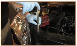
**10.** Remove (2 )10mm fan shroud to radiator bolts. Remove the overflow reservoir and the water line near the radiator cap.
