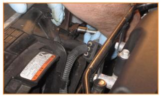
**11.** Unplug the radiator fan; remove the wiring harness from the fan shroud.
