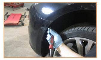
**6.** Remove the (8) plastic screws for the front bumper on the radiator support.
