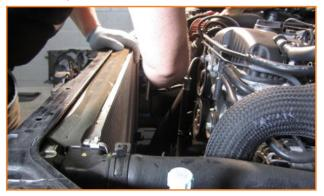
13. Reinstall the (2) 10mm bolts for the fan shroud.
