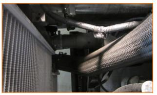
**16.** Remove (4) 10mm bolts holding the radiator to the intercooler. (2 on each side of the radiator)
