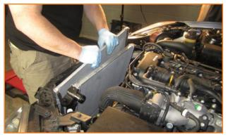
18. Disconnect the Intercooler charge piping.
