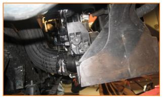
**17.** Pull up on A/C condenser to remove from the radiator holsters and remove radiator from the vehicle. Do not remove the A/C condenser from the vehicle, as this will require you to recharge the A/C system once completed.
