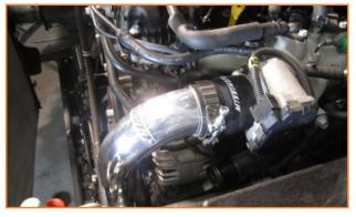
**6.** Install the Mishimoto coupler onto the turbo, install upper and lower hot-side piping, and install t-bolt clamps onto the hot side.
