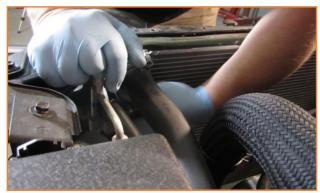
13. Pull off insulator strip on top of radiator.
