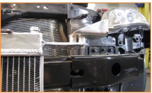
**9.** Reinstall air dams onto the front of the vehicle and reinstall the radiator from the top of the vehicle. Lift up on A/C condenser to allow condenser to sit into the radiator holsters.
