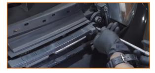
9. Lean the top of the bumper back far enough to reach behind it. Pull out the blinker bulbs from inside the bumper.
