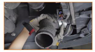
Loosen the clamp and release the clip from the hot-side coupler/hose, and then remove it. (1x worm gear clamp, 1x spring clip)
