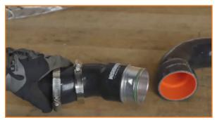
48. Install the hot-side coupler to the intercooler and pipe. Align the protrusions on the adapter with the notches on the pipe. Then tighten the clamps and make sure the clip engages the barbs on the adapter. (2x worm gear clamp, 1x spring clip)
