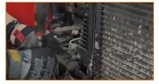
28. Separate the intercooler from the radiator. There is a bolt at each corner of the radiator. (4x T30 torx bolts)
