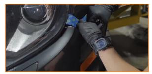
8. Remove the last two bolts securing the top of the bumper. (2x T25 torx)
