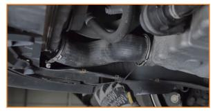
5. Remove the bolts in each wheel well that hold the bumper. (10x T25 torx bolts)
