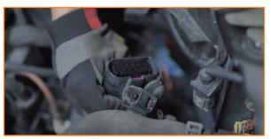
17. Separate the hood latch connector found under the headlight support bar.
