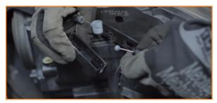
Remove the bolts at the side of each headlight. (6x T25 torx bolts)
