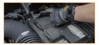
16. Unplug the yellow and red crash sensors as well as the headlight. Slide the red tab down and pull the connector out of the harness.
