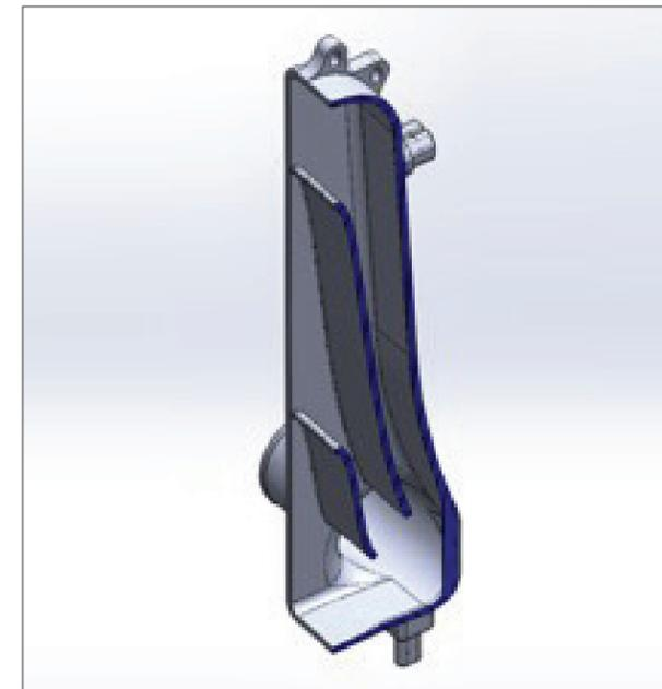
FIGURE 3: Two internal air diverters are integrated into the hot-side end tank.
