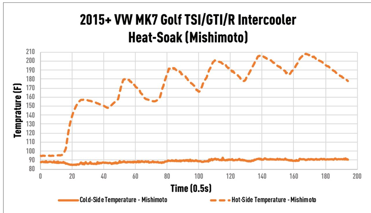
FIGURE 8: Heat-soak test.
