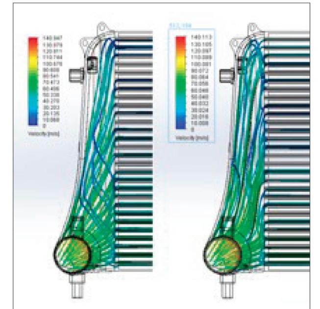
FIGURE 4: CFD comparison results, before and after the air diverters are added into the design.
