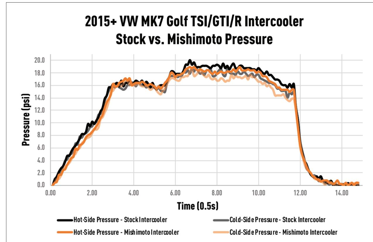
FIGURE 6: Pressure drop comparison.
