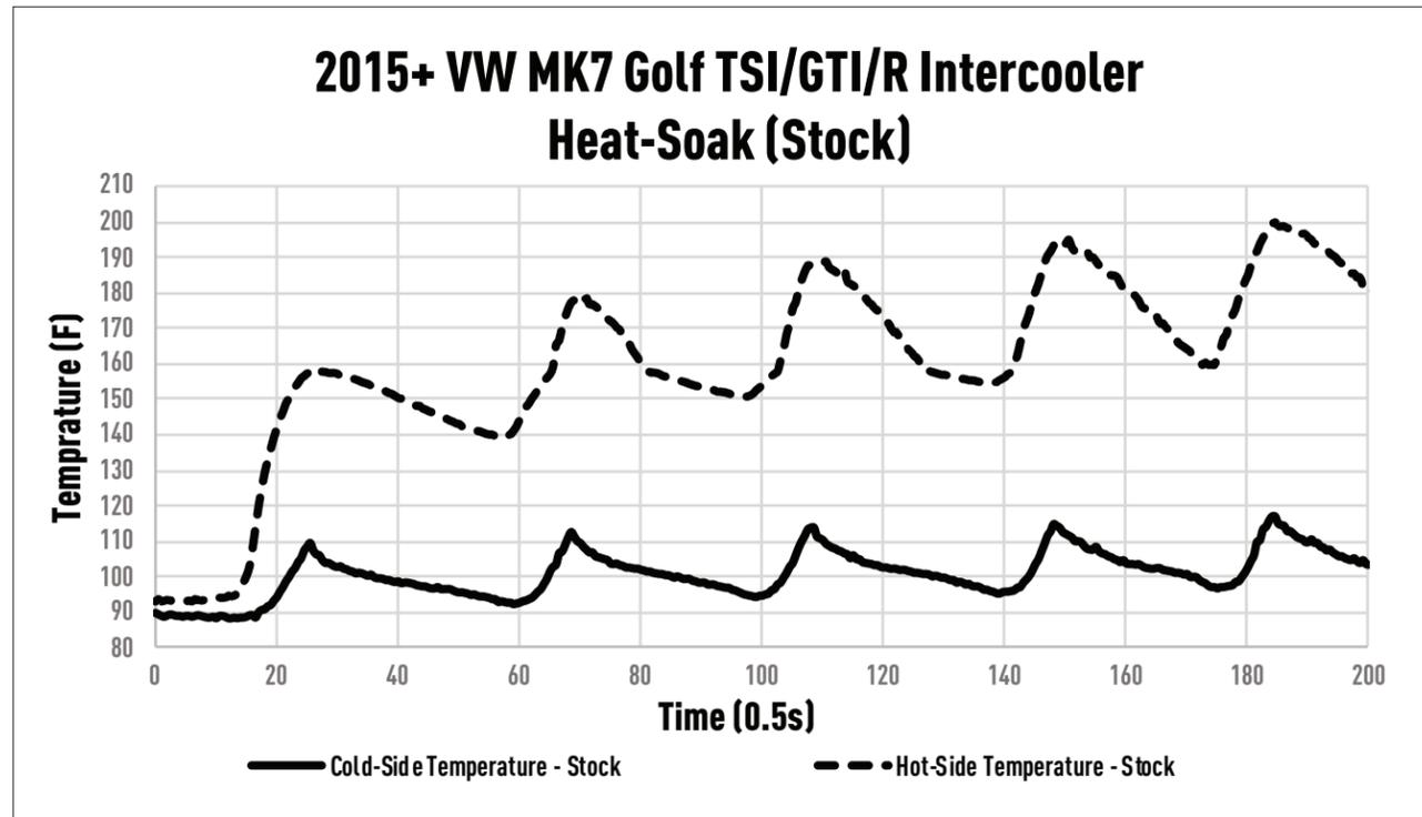
FIGURE 7: Heat-soak test.
