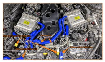
**06.** Loosen 8x hose clamps from the inlet and outlet air couplers on both intercoolers.
