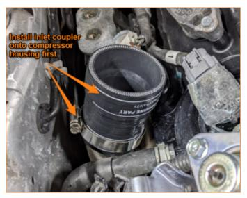
**16.** Place inlet of intercooler into inlet couplers first.
