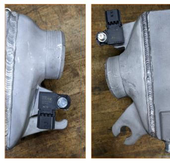
**14.** Install outlet couplers onto intercoolers with clamps loosely in place.
