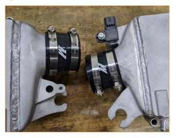
**15.** Install inlet couplers with clamps onto turbo compressor outlet flange first, leaving clamps loose.
