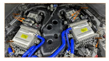
**07.** Remove the hold-down bolts and unplug boost pressure sensor from both intercoolers.
