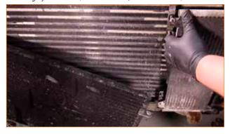
08. Remove the two bolts that secure the stock intercooler to the radiator support. Remove the intercooler from the vehicle, taking care not to damage the AC condenser or transmission cooler. (2x 10mm bolts)
