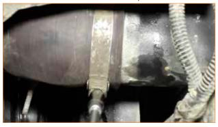
06.To make room for the larger intercooler, you will need to bend the body panels near the intercooler inlet and outlet. Locate the body panels, then bend the front edges of these panels upward. Tip: A pair of vice grips makes this job easy.
