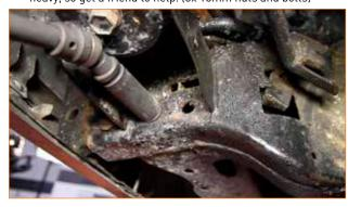
03. Remove the seven bolts that secure the radiator support beam to the vehicle. There are three bolts on either side of the support beam, and one on the back of the beam just behind the hood latch. Lift the support beam off the vehicle and move it out of the way, allowing it to hang on the hood-release cable. [7x 13mm bolts]
