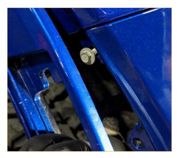
**06.** Remove 3x bolts securing the bumper fascia support (black plastic structure) to the frame, along the intercooler's underside. Repeat steps 3–6 on the other side.
