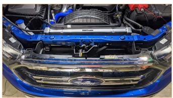
02. Remove the radiator grille. Loosen the two bolts at the top of the grille, then pull forward to disengage the tabs along the bottom and side edges.
