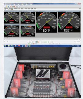
Figure 4: PLX sensor modules were used to monitor engine pyrometers.
