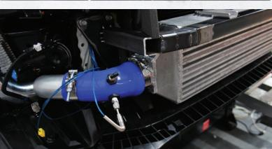
Figure 3: Mounting location for Inlet temperature sensor, which reads approximately 10 times per second.
