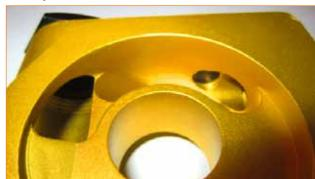
6. Notice that no Teflon® tape is inside the npt port area.
