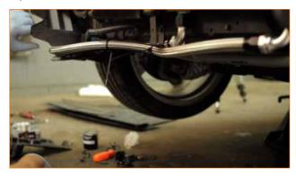
**6.** Once all the lines are tight you can reinstall the oil filter.
