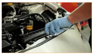
**5.** Remove the four pop clips from the inside of the fender on each side of the car. One pop clip is behind the corner marker light.
