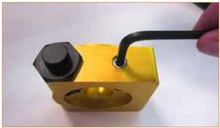
5. Remove any excess Teflon® after tightening.
