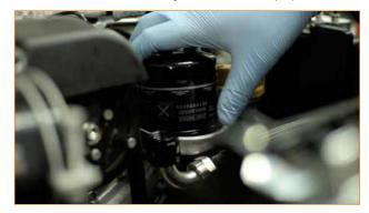
**7.** Install the Mishimoto sandwich plate. Make sure to lubricate the O-ring with oil to create a proper seal.
