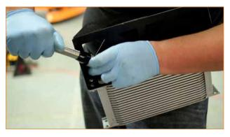
**3.** Install the Mishimoto oil cooler and feed the oil lines into the engine compartment.
