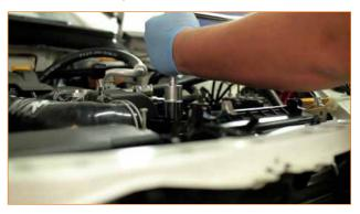
**10.** Install the oil lines onto the sandwich plate. Tighten down all the oil line fittings.
