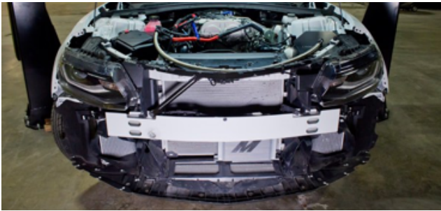
FIGURE 1: The Mishimoto oil cooler was mounted in front of the lower grille opening for optimal airflow.
