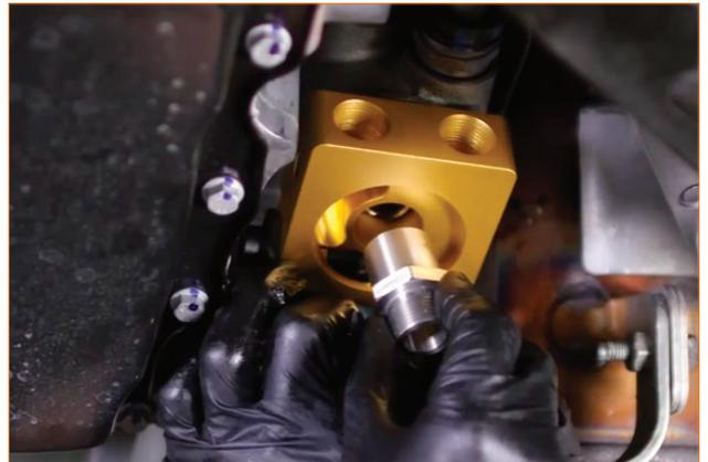
41. Install the two provided fittings to the sandwich plate, and tighten them completely. (2x fittings)
