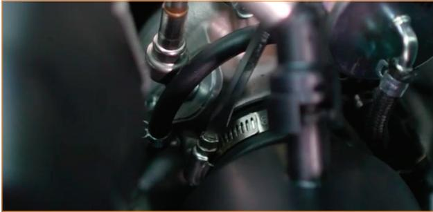
03. Disconnect the CCV hose from the intake by sliding the locking tab over and pulling the hose off the port.
