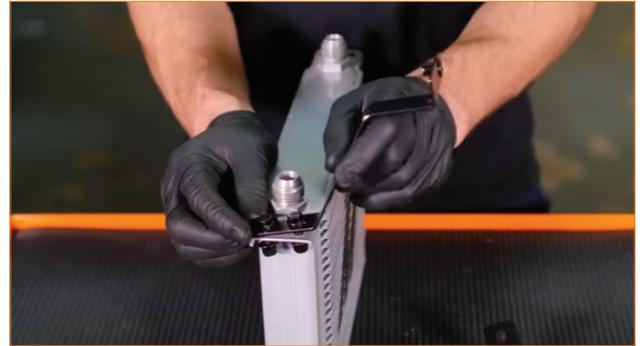
33. Locate the angled bracket in your kit. Attach this bracket to the driver-side of the oil cooler with the provided hardware, but do not fully tighten it yet. (2x 10mm bolts, 2x Nyloc nuts)
