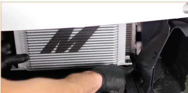
38. Now that all the brackets are attached, go back and tighten all the bolts that secure the cooler to the brackets.
