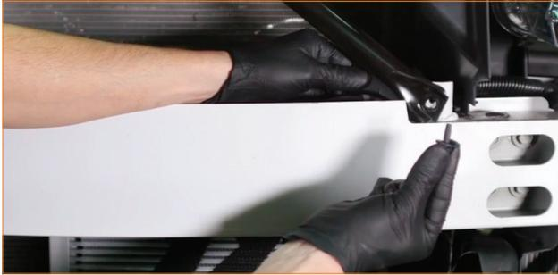
36. Align the driver-side bracket with the hole in the crash bar, and secure it with the provided bolt and washer. (1x 10mm bolt, 1x plastic washer)
