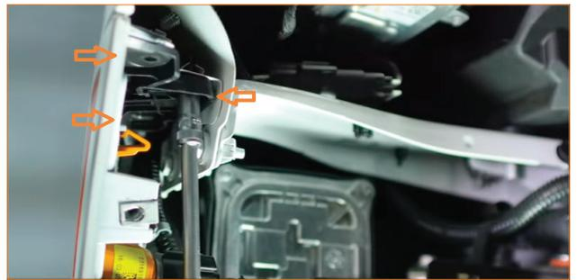
16. Pull the upper corner of the bumper away from the fender to release it from the vehicle.
