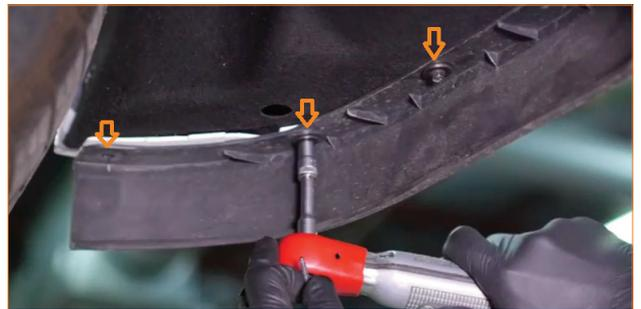
09. Remove the eight screws that secure the lower edge of the bumper. (8x 7mm screws)
