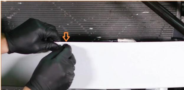
37. Align the lower bracket in your kit with the holes in the air diverter, and reinstall the two pop-clips to secure it. (2x pop-clips)
