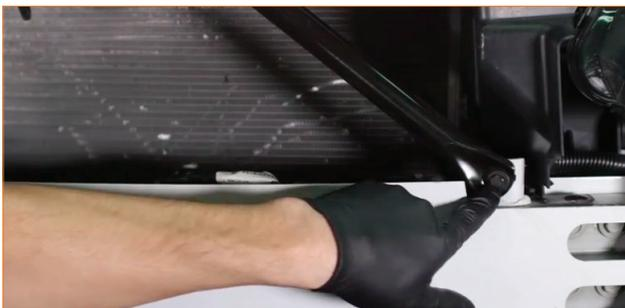
32. Locate the large bracket with the threaded insert in your kit. Attach this bracket to the passenger side of the oil cooler with the provided hardware, but do not fully tighten it yet. (2x 10mm bolts, 2x Nyloc nuts)
